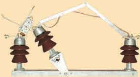
11/22/33 KV Outdoor triple pole Three insulator per pole tilting type, Gang Operated Air Break Switch Suitable for horizontal / vertical mounting with complete operating mechanism. Test as per IS-9920 / 1985
