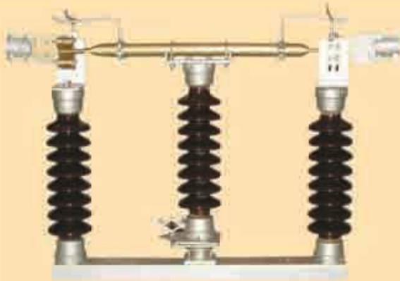
33 KV Outdoor triple pole Three Solidcore insulator per pole Rotating type, Isolator Suitable for horizontal mounting with complete operating mechanism. Test as per IS-9920 / 1985
