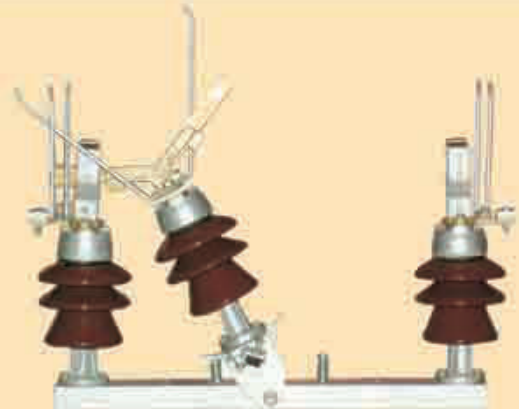
11/22/33 KV Outdoor triple pole Three insulator per pole tilting type, Gang Operated Change Over Switch Suitable for horizontal / vertical mounting with complete operating mechanism. Test as per IS-9920 / 1985
