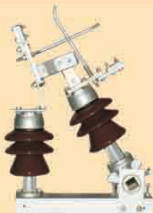
11/22/33 KV Outdoor triple pole Two insulator per pole tilting type, Gang Operated Air Break Switch Suitable for horizontal / vertical mounting with complete operating mechanism. Test as per IS-9920 / 1985
