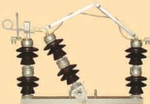
22/33 KV Outdoor triple pole Tilting type, Gang Operated Air Break Switch with Double Stack of Insulator Suitable for horizontal / vertical mounting with complete operating mechanism. Test as per IS-9920 / 1985
